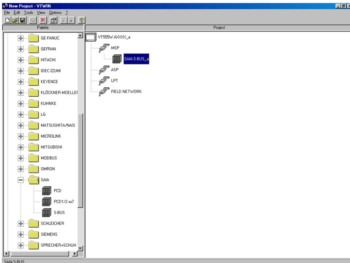
The program is checking if a driver/unit can be connected to a port of the terminal. If this is not allowed, the connector doesn't get blue.
