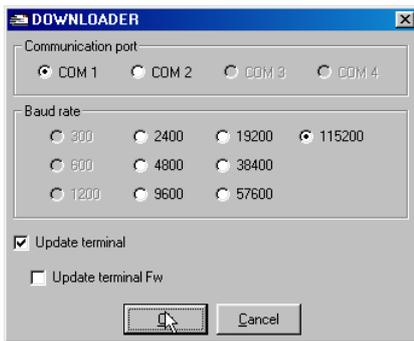
The baud rate you select has nothing to do with the baudrate used later for the communication with the PLC, so try with 115200.
