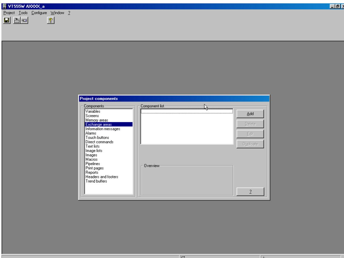
The exchange areas in a standard PCD are one or more registers, for xx7 a DB. The length of the buffer is always indicated in words (1 word = 16 bit), so two words occupy a register. Consult the table below to know what exchange area size has to be defined:
