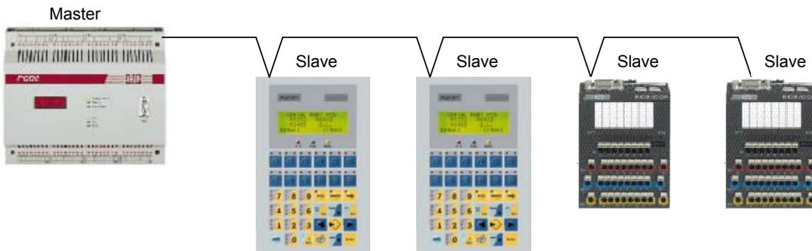
The PCD contains a driver per slave terminal which leads to long cycle times which means long reaction times on the whole DP network (up to 16 ms per terminal). Therefore the use of terminals as DP slaves is not recommended.
