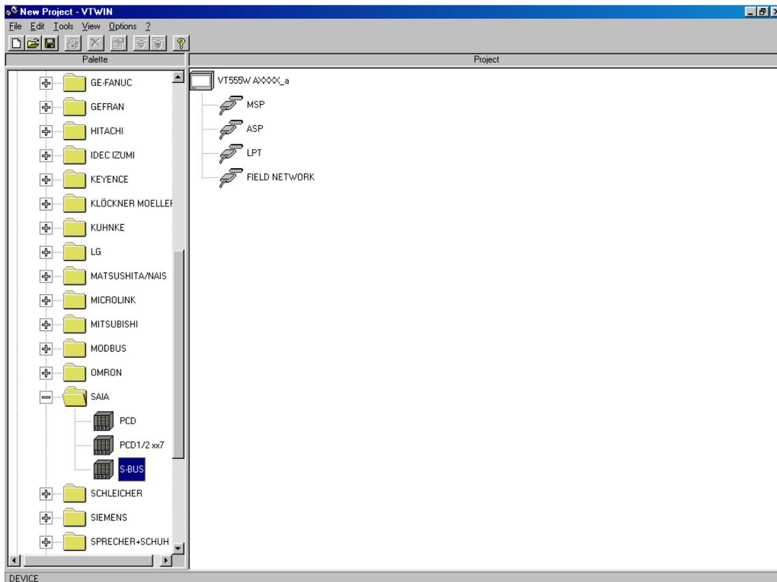
Select the S-Bus Driver with the left mouse button, keep the button pressed and drag the driver to the MSP port of the terminal:
