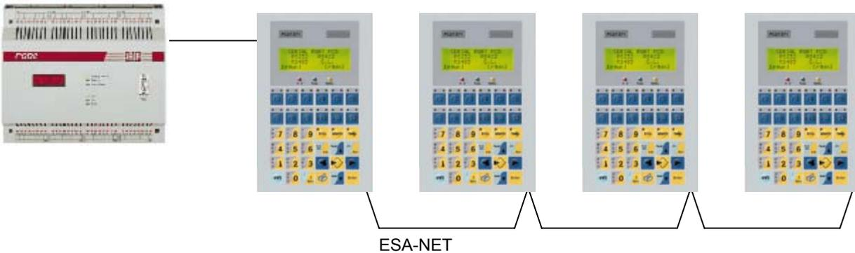
Remark: The ESA-NET server terminal (connected to the PLC) must have two ports. A good choice are the PCD7.D760 touchscreen terminals for ESA-NET networks as they can be client and server and are not very expensive.
