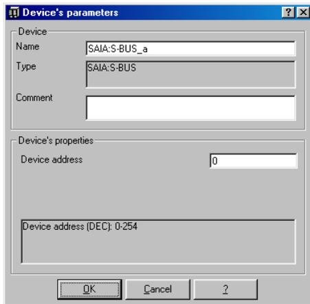
This choice is very important since the addresses have to match with the configuration of the PCD or no communication will be possible.
