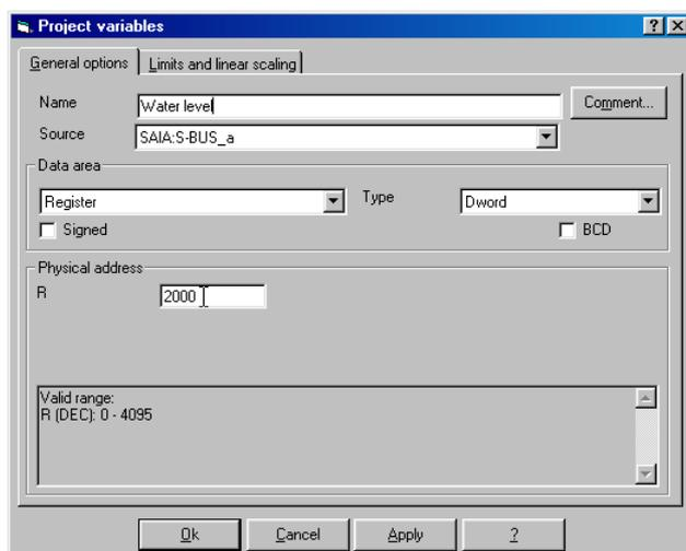
Define limits and a linear scaling if required, confirm with OK:
