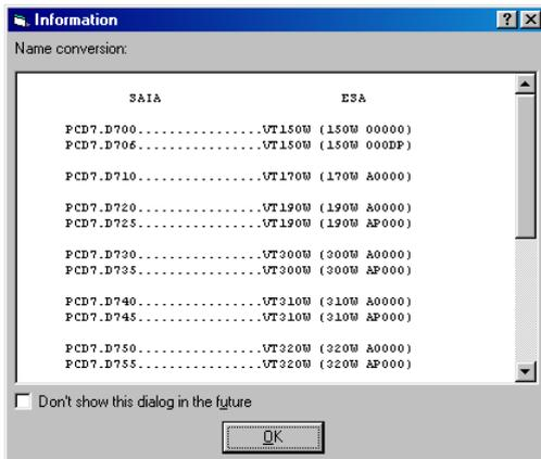
Select the terminal to program (or select the project under recent if you continue an existing project) A PCD7.D760 which is equivalent to a VT555W AXXXX is selected for this example, confirm with OK.
