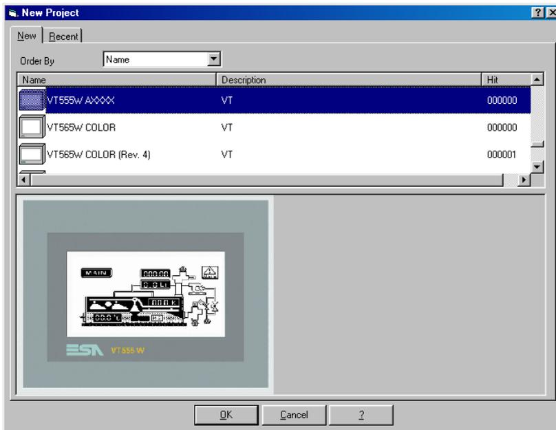
The terminal you selected is shown as follows and you are able to select the PLC the terminal is connected to within the list at the left hand side.
